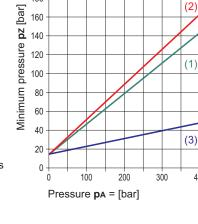
Minimum opening pressure pz at pressure pa (pb = 0 bar)
